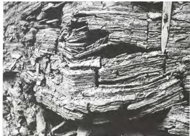
Figure 4. An example of the weathering of the laminated clays /Krakowiec clays/. Machów.
