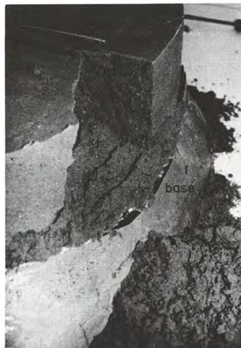
Fig. 8. Toppled and sheared off tower shaped block in a model test (slab: sand, base: silicon-caoutchouc)
