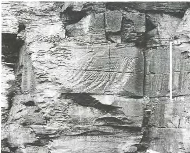
Figure 2. Lamination and discontinuity-surfaces of the joint type in Krakowiec clays. Machów.
