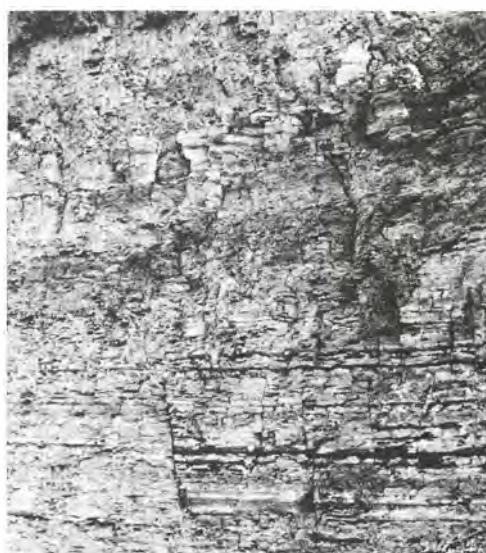
Figure 5. Typical profile of the weathered zone in Krakowiec clays. Machów.
